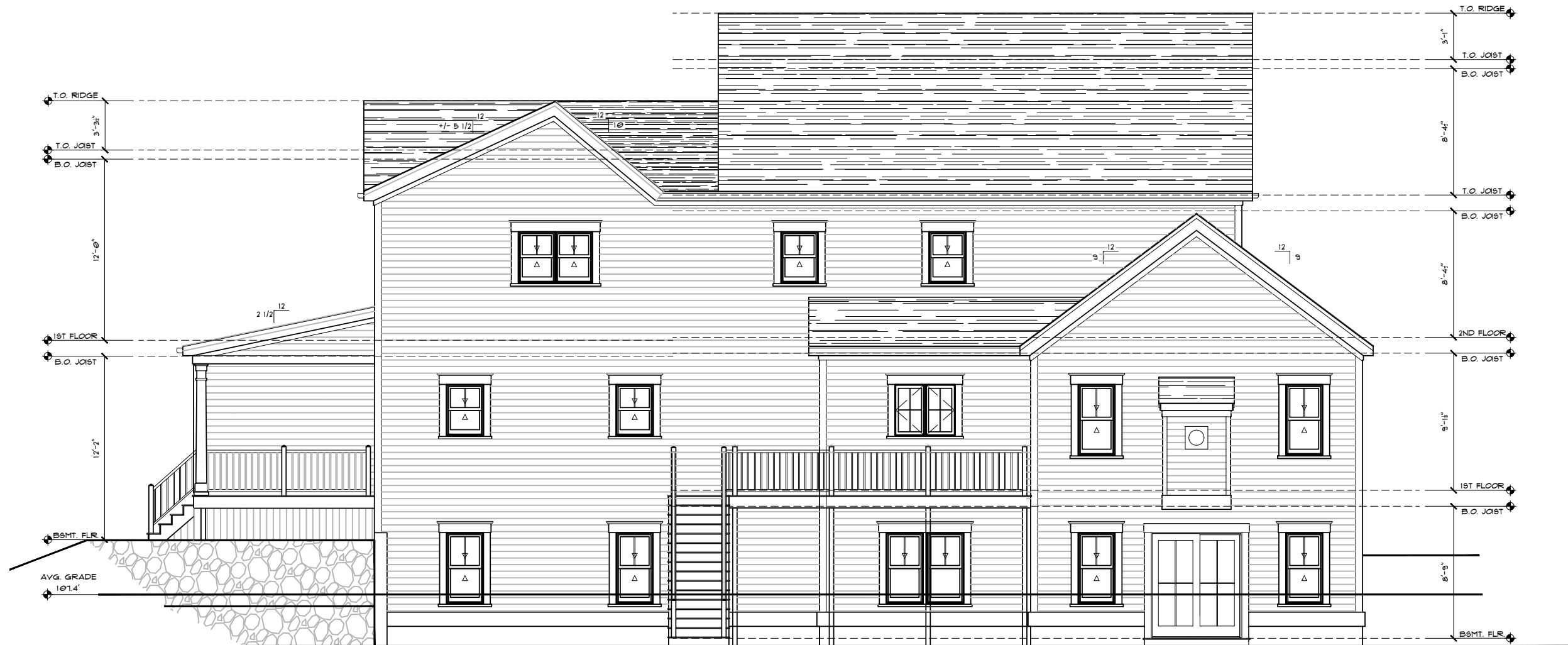
REAR ELEVATION LOT 5 SCALE: 1/4"=1'-0"
